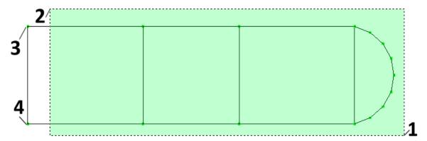
When you get the message *Specify second point of mirror line,* click on the joints at points 3 and 4 as shown in the picture above.
