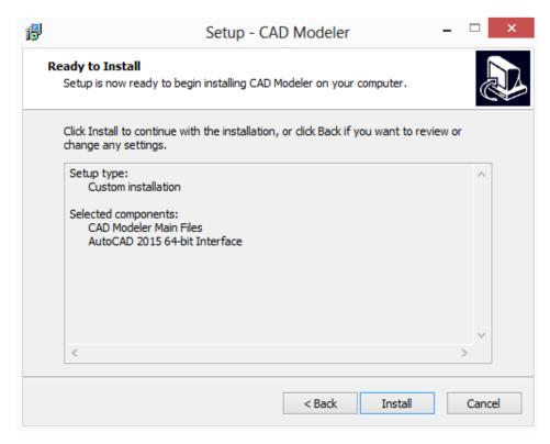
CAD Modeler is installed in the same installation directory with GT STRUDL, under the sub-directory "CADModeler". For example, "c:\Program Files (x86)\GTStrudl\2015\CADModeler" is a typical CADModeler installation directory.
