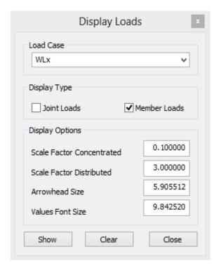
The "Display Loads" form appears where you can select the desired Load Case, the Scale factor for Concentrated or Distributed Member Loads, Arrowhead Size and the Font Size. The "Show" button displays the load arrow, and "Clear" button erases them.
