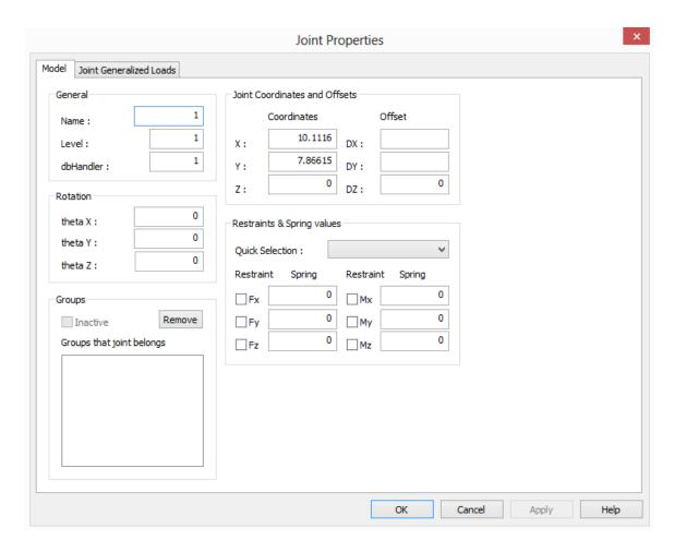
The "Joint Properties" form appears, and at the "Model" tab you can enter the Name of the Joint (up to 8 characters) the Level that the joint belongs (optional), the theta rotation angles for rotated support joints, the *Groups* that the joints belongs to, the coordinates of the joint in the current unit system, the restraints of the joint and the spring values.
