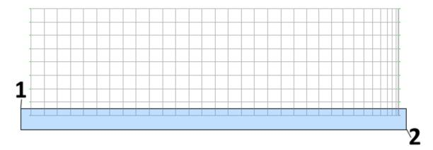
All the shell elements located in the bottom of the tank are now selected and added to group "Bottom".
