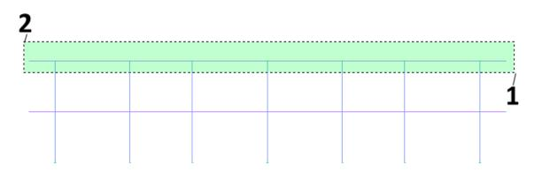
In order to Specify base point or [Displacement] < Displacement>: click ANYWHERE on the screen. It makes no difference where you click since relative coordinates will be use to define the displacement.
