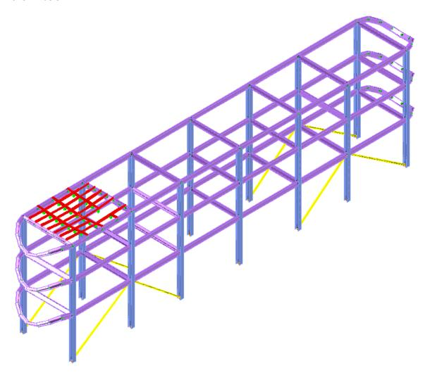
Repeat and select PL as the Load Case and the deformed structure appears as shown in the following image:
