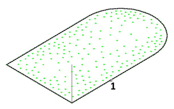
When the prompt message *Select Extrude Direction Curve (Line or Arc)* appears, click on the line that you have created in a previous step, as shown in the picture below (Click #2).
