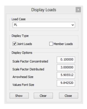
The "Display Loads" form appears where you can select the desired *Load Case*, the *Scale Factor* for Joint Loads, *Arrowhead Size* and the Font Size. The "Show" button displays the load arrows, and the "Clear" button erases them.
