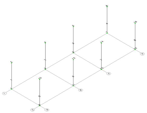
**Step #9.** Start entering the beams, along X axis, by clicking on the icon Generate and the prompt message *Starting Point (x,y,z)* appears, asking you to enter the coordinates or click on a specific point on screen. Click on Joint 2 at the top joint of column 1 at position A-1.
