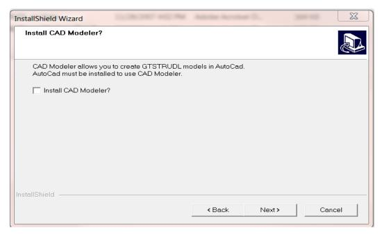
CAD Modeler Installation can also be launched independently, after GT STRUDL installation, by executing the file "CADM\_setup.exe" which is located in the CADModeler folder in the GTStrudl
