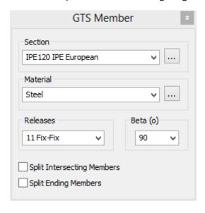
Select *IPE120* as the cross section and make sure that Material is set to *Steel*, Releases to *Fix-Fix* and Beta angle is *90*.
