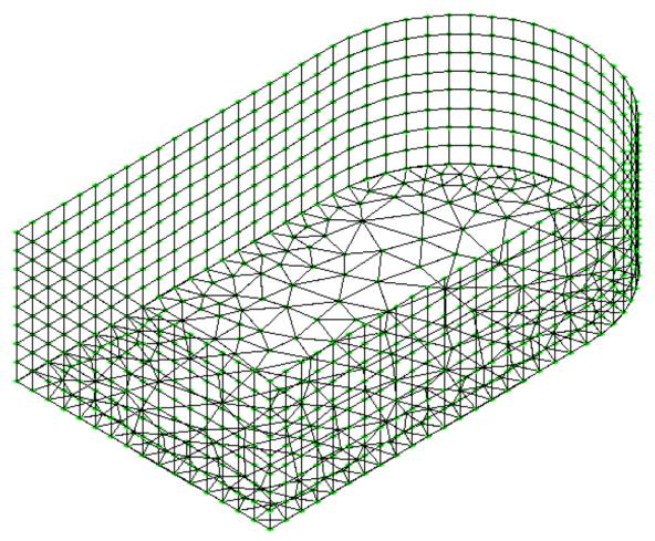
**Step #59.** Check for duplicate joints: Since both meshing functions described above generated joints along the polyline, pairs of joints having the same coordinates exist in the model and they have to be merged together. In order to check for joints having the same coordinates, click on the icon Locate Duplicates under the Joints panel.
