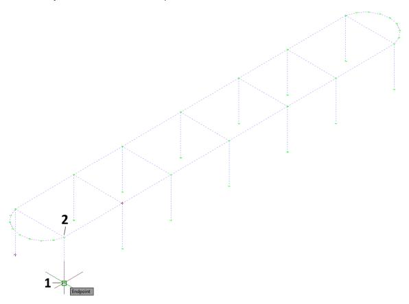
In order to *Specify base point or [Displacement/mOde] <Displacement>*, click at the base of any column such as point 1 in the picture above.
