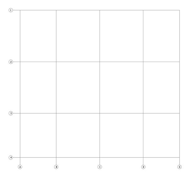
You can also change the properties of an existing grid by expanding the "Levels" tab and selecting the ribbon icon "Change Grid, or from the menu "GTS Modeling>Grid>Change" or by typing GTSGridChange at the command prompt, and then selecting the Grid to be edited.
