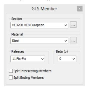
This dialog helps you to quickly select properties for the members that are going to be entered. Select *HEB320B* as the cross section for the columns. Make sure that Material is set to *Steel*, Releases to *Fix-Fix* and the Beta angle is *0*. There is no need to close this dialog manually.
