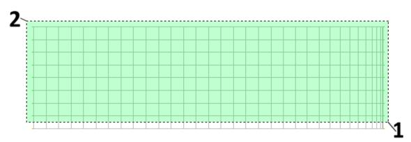
All shell elements located in the wall of the tank are now selected and added to group "Wall".
