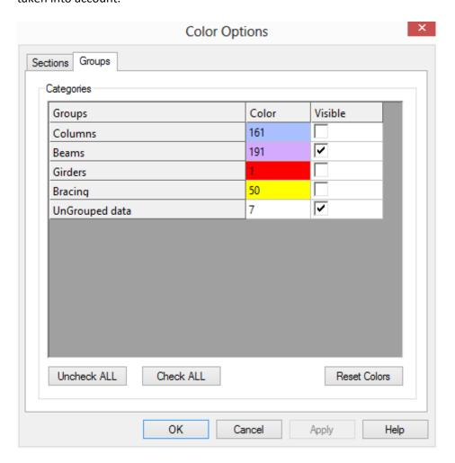
Note, that if the "Sections" tab is active when pressing "OK", then the colors will be selected according to the "Sections" tab. If the "Groups" tab is active when pressing "OK", then the colors will be selected according to the "Groups" tab.
