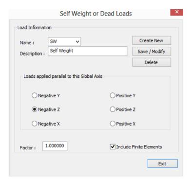
The "Self-Weight" form appears where you can define the global direction of the self-weight and a factor (default = 1.0) for the self-weight and also define if the self-weight of finite elements will be taken into account or not.
