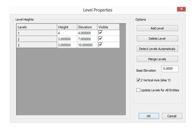
After defining Levels, you can switch between levels by either using the "Visible" checkboxes from the Level Properties form, or using the Higher Level and Lower Level icons in the ribbon area. You can also type GTSLevelUp and GTSLevelDown at the command prompt.
