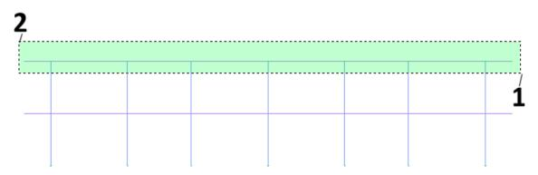
In order to Specify base point or [Displacement] < Displacement>: click ANYWHERE on the screen. It makes no difference where you click since relative coordinates will be use to define the displacement.
