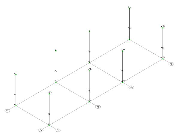
**Step #9.** Start entering the beams, along X axis, by clicking on the icon  $\checkmark$  Generate and the prompt message *Starting Point* (x,y,z) appears, asking you to enter the coordinates or click on a specific point on screen. Click on Joint 2 at the top joint of column 1 at position A-1.
