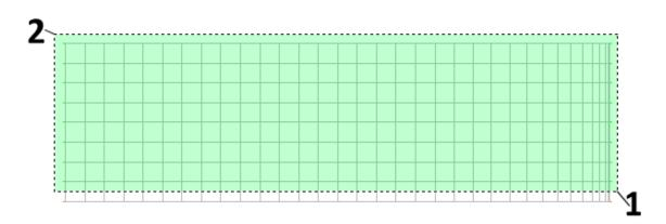
All shell elements located in the wall of the tank are now selected and added to group "Wall".
