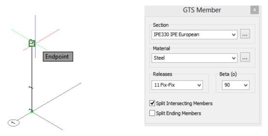
Select *IPE330* as the cross section and make sure that Material is set to *Steel*, Releases to *Fix-Fix* and the Beta angle is *90*. You have to set the Beta angle equal to 90 degrees in order to orientate
