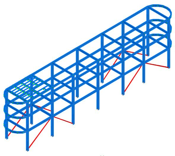
**Step #54.** Display Member Diagrams: Click on the icon Frame to switch back to the wireframe view. Click on Diagrams (ribbon tab "GTS Display").
