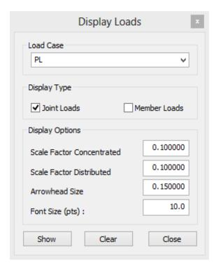
The "Display Loads" form appears where you can select the desired *Load Case*, the *Scale Factor* for Joint Loads, *Arrowhead Size* and the *Font Size*. The "Show" button displays the load arrows, and the "Clear" button erases them.
