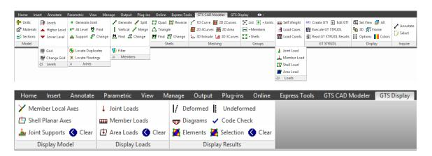
If AutoCAD menu is visible, then CAD Modeler commands can be accessed from Menu Area at the top of the window by selecting GTS Modeling or GTS Display
