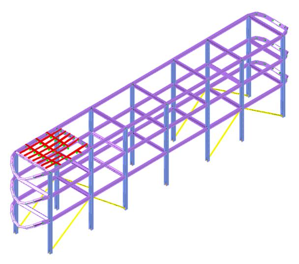
Repeat and select PL as the Load Case and the deformed structure appears as shown in the following image:
