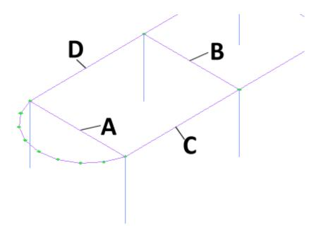
**Step #28.** Place girder members at the top level: Click on the icon Generate and click on joint located at the point 1 of the following image.
