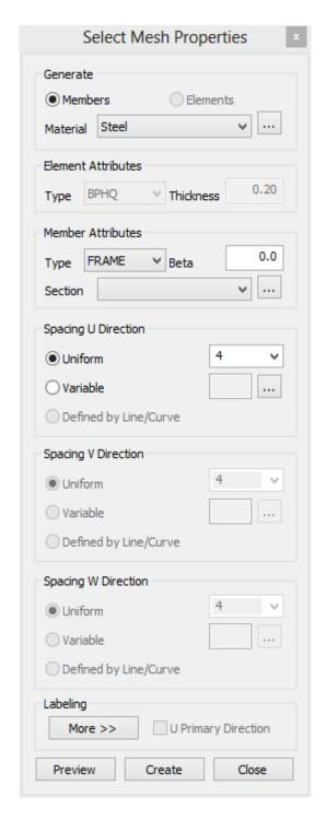
After selecting the AutoCAD linear entity the Mesh Properties dialog appears, where you can define:
