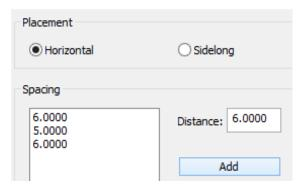
Then, click on *Sidelong* in the *Placement* area to enter the spacing in the Y direction, and enter 5 and *Add*.
