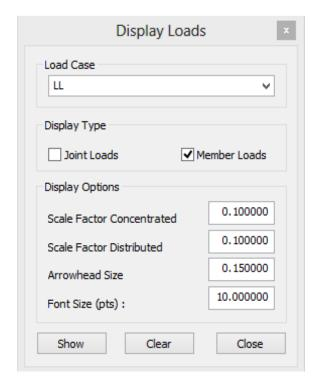
The "Display Loads" form appears where you can select the desired Load Case, the Scale factor for Concentrated or Distributed Member Loads, Arrowhead Size and the Font Size. The "Show" button displays the load arrow, and the "Clear" button erases them.
