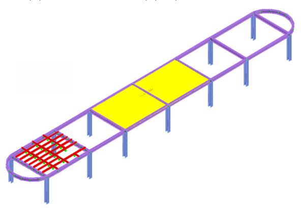
Press Clear to remove the solid hatch pattern and then <u>OK</u> to store the area load AL3.
