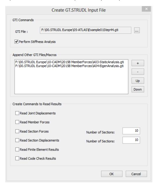
Moreover, you can append additional GTI Files or Macros at the end of the GTI file of the model. For example, additional GTI files may include static or dynamic analysis commands, result output commands or member design commands.
