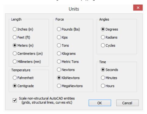
You can change the Units any time during working in CAD Modeler. Moreover, you can choose if the non-structural AutoCAD entities, such as grids, structural lines, curves, polylines, etc will be scaled together with the structure whenever you change the length units.
