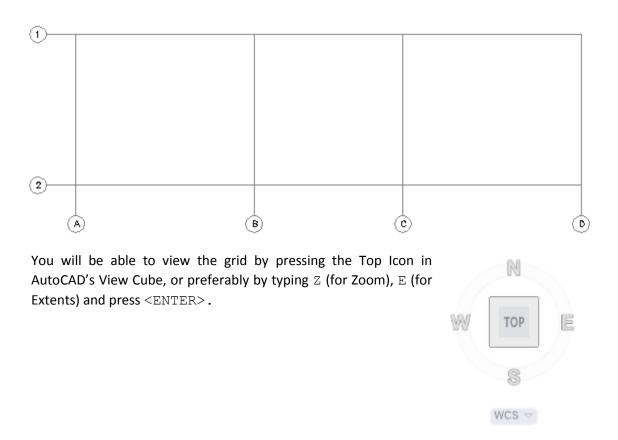
Note: In order to be able to snap at the intersection of the grid lines, while placing columns, make sure that the AutoCAD's Object Snap is ON, and the Intersection mode is enabled.
