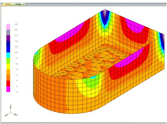
**Step #26.** Read Results from GT STRUDL: Click on the icon Read GT STRUDL Results and the Read GT.STRUDL Results dialog appears. Check the options "Read Joint Displacements" and "Read Finite Element Results" as shown below and press OK.
